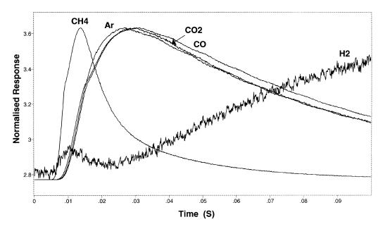
FIG. 1. The normalised responses of CH<sub>4</sub>, Ar, CO<sub>2</sub>, CO, and H<sub>2</sub> as a function of time when pulsing CH<sub>4</sub>, CO<sub>2</sub>, and Ar at t=0 s and 700°C. Note that all signals have been normalised to the largest response, which was that of CO<sub>2</sub>.
