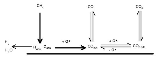
FIG. 4. A scheme of the reaction pathway of the over Pt/ZrO<sub>2</sub>.
